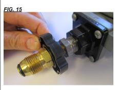
4. Insert the POL stem into the cylinder valve. Push the spring loaded hand wheel up against the threaded nut. Turning counter clockwise, thread the POL nut into into the container valve using the hand wheel. Firmly tighten. See Fig. 16.
